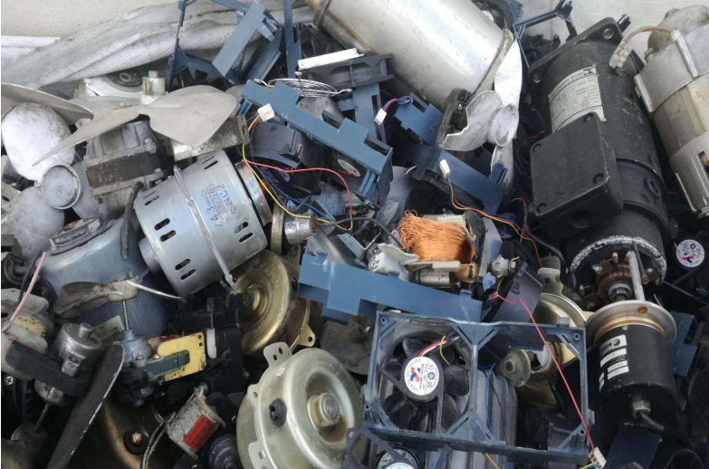
DESCRIPTION: electric motors / coolers from WEEEs.
