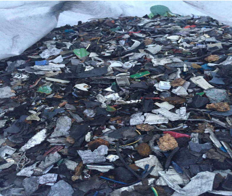
DESCRIPTION: Plastic from the recycling from small electrical appliances in big bags.
